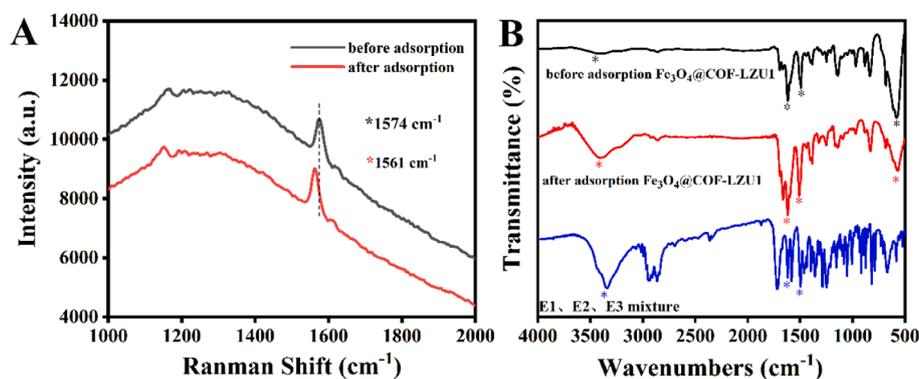
Fig. 4. (A) Raman spectra and (B) FT-IR before and after  $\text{Fe}_3\text{O}_4@\text{COF-LZU1}$  adsorbed three estrogens.
