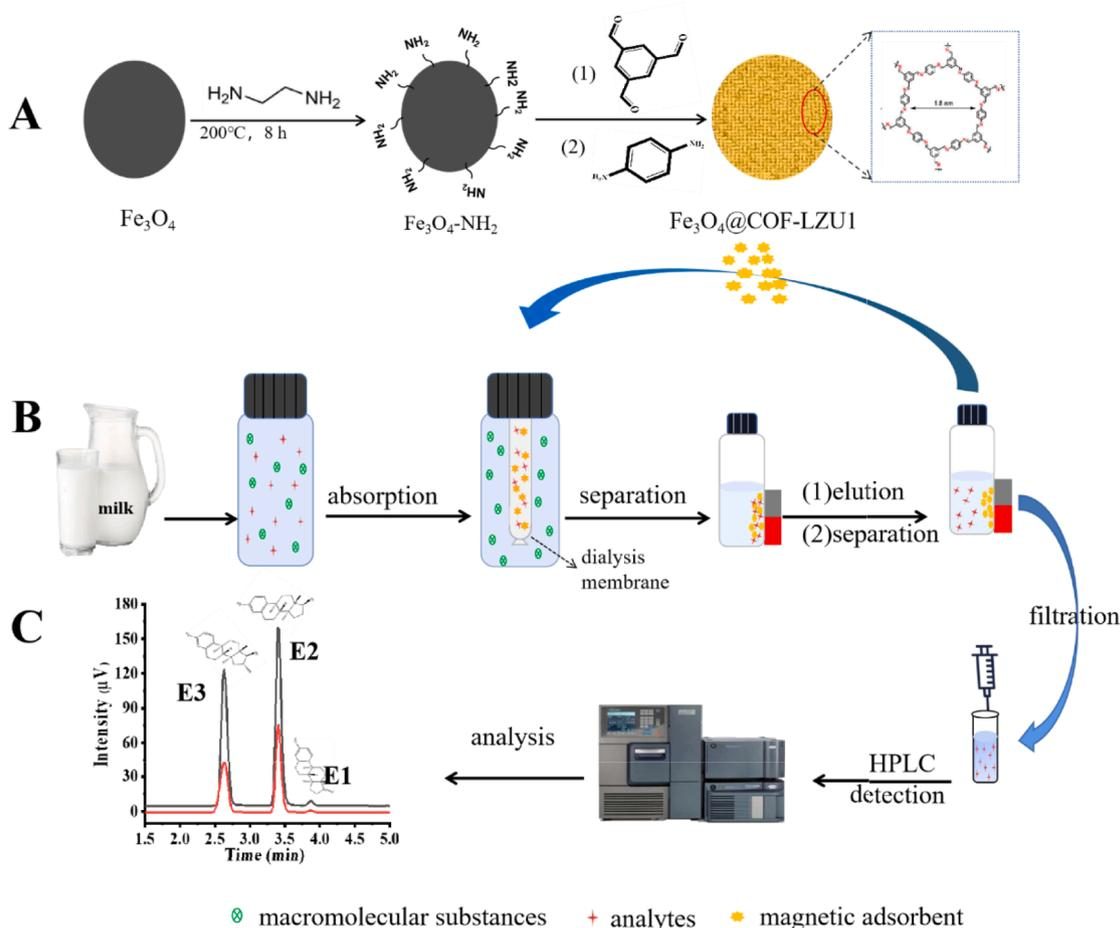
Fig. 1. Schematic diagram of (A) preparation of  $\text{Fe}_3\text{O}_4@COF-LZU1$ , (B) membrane separation MSPE process, and (C) HPLC-FLD detection of estrogens.
