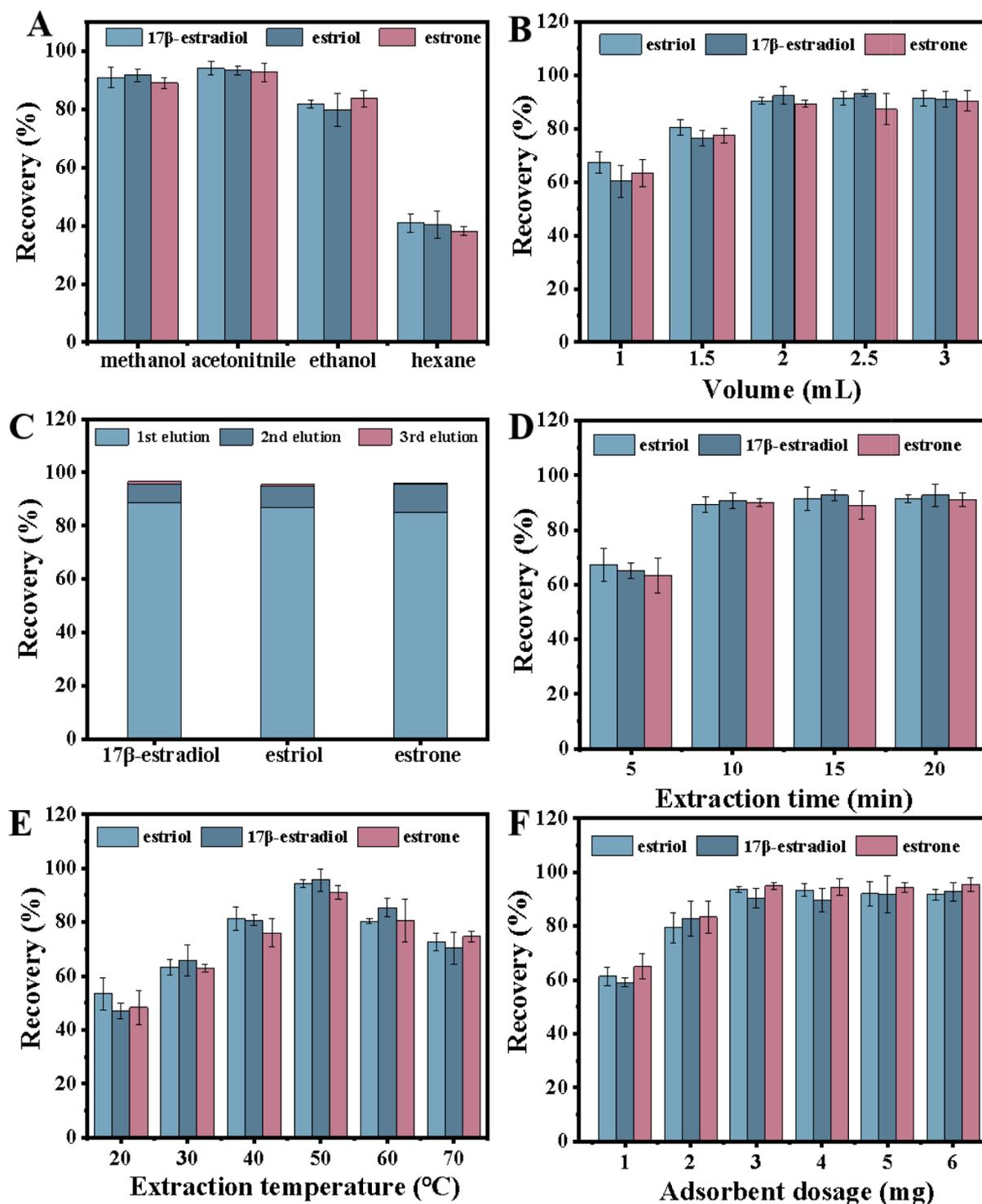
**Fig. 3.** Effect of (A) desorption solvent, (B) desorption solvent volume, (C) elution times, (D) extraction time, (E) extraction temperature, and (F) adsorbent dosage on extraction efficiency of estrogen.
